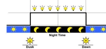
Turn-On voltage (Adjustable): 5V(12Vsystem),delay10min.
