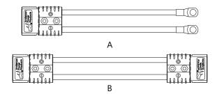
Anderson connector is used on the DC input side of wall mounted battery series. The specific connections are as follows:
